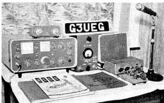
G3UEG's station, from where the Slow Morse course signals emanated, showing all the equipment with the exception of the a.t.u. which couples into a 260 ft. long end-fed wire, 35 ft. high. On the right hand side is the fully automatic key and a Vibroplex paddle which gives a speed range of 6 to 18 words per minute with correct timing and spacing.
